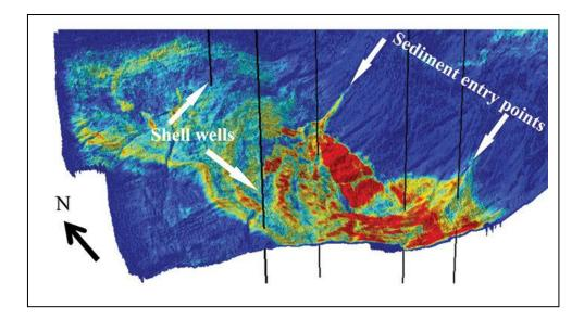
[Figure 3 – amplitude and seismic drape of Sea Lion field]
