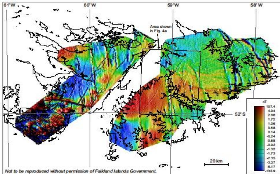
**Fig. 2.** Aeromagnetic image of the Falkland Islands, based on a residual field calculated by subtracting a 0.5 km upward continuation from the total magnetic field. Colour shaded-relief image with equal colour area and illumination from the west. The survey comprised N-S flight lines at a typical spacing of 0.5 km and E-W tie lines at a spacing of 5 km; the flying height was 120 m above terrain.
