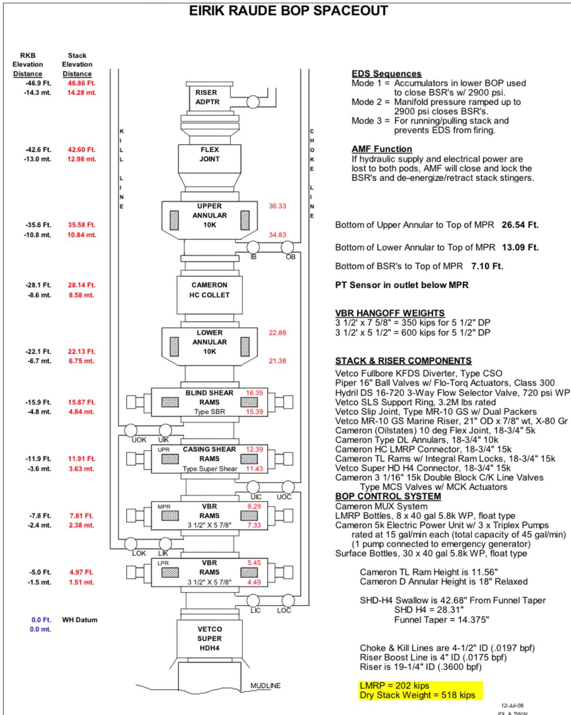
Figure 10: Eirik Raude Blow Out Preventer Spaceout Diagram
