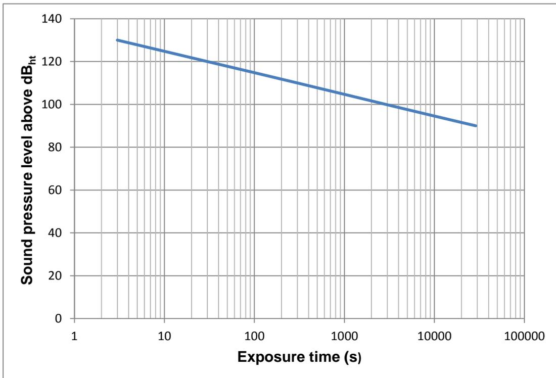
Figure 50: Comparison of sound pressure level and duration for the same cumulative noise dose (from Nedwell et al., 2007)
