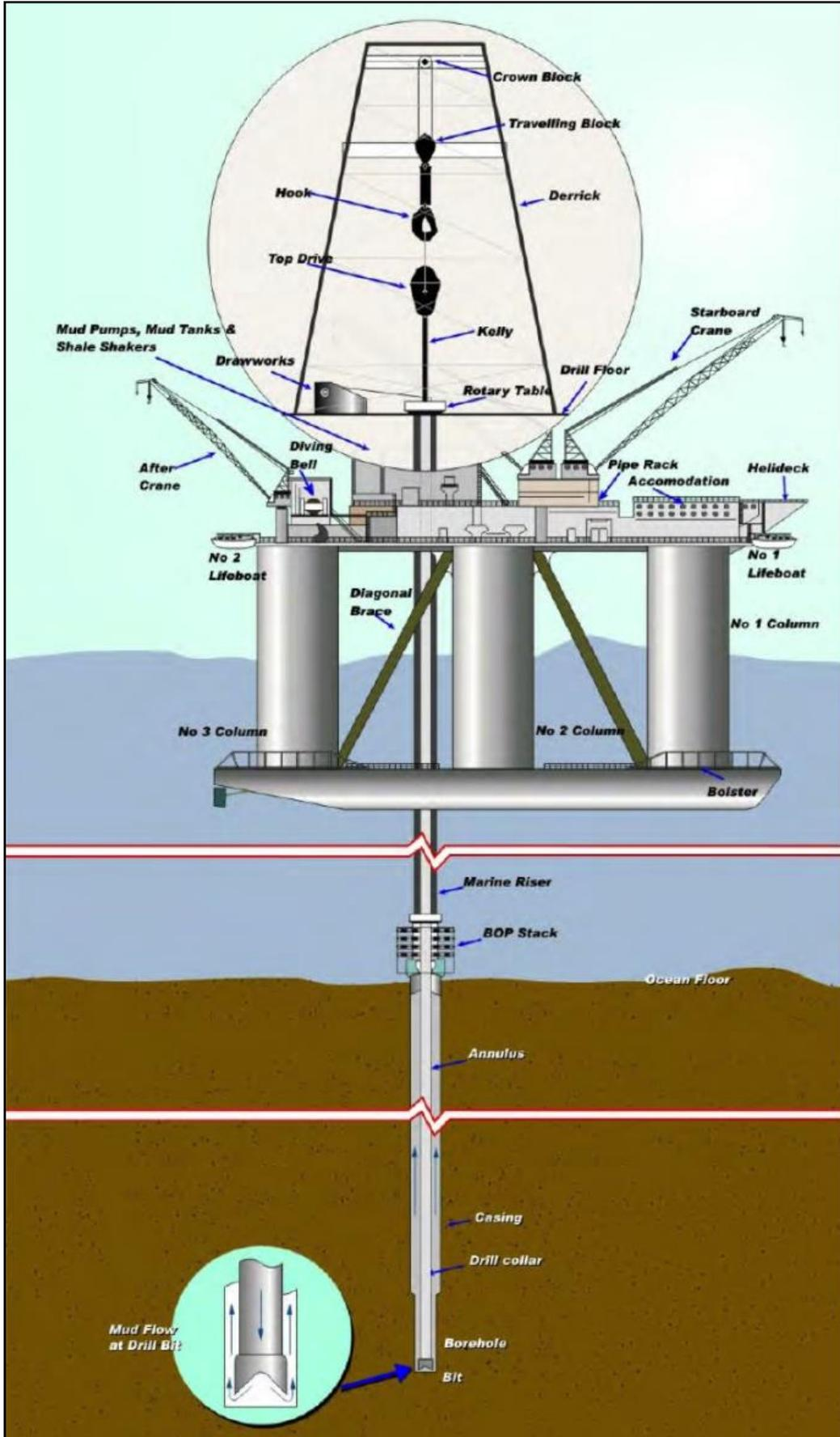
Figure 8: Conventional rotary drilling system diagram
