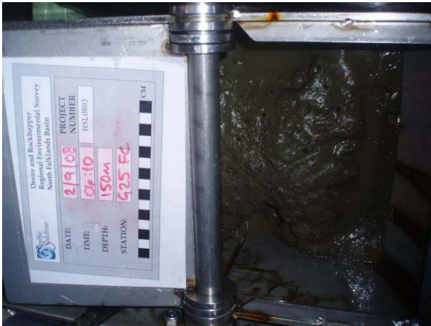
G25 Depth 150 m Muddy fine sand with gravel and coarse sand fraction
