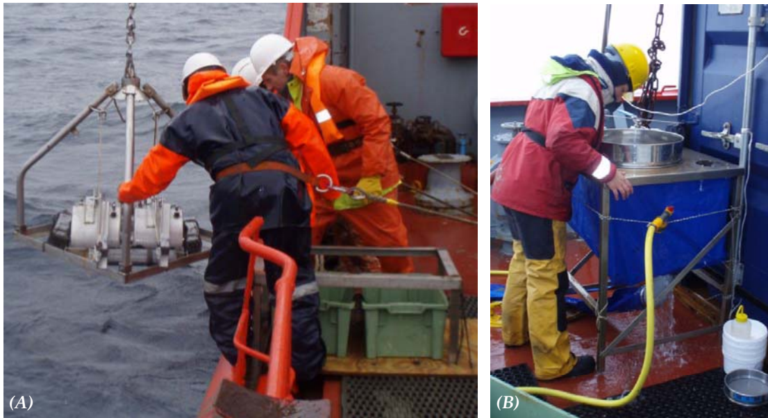
(A) Deployment of the unique Benthic Solutions Double Grab (0.2m 2 ). Personnel all wear safety lines. (B) Benthic samples were processed by Wilson Autosiever over 500µm. (C) Decapods Peltarion spinosulum found in one sample. (D) Example grab samples taken at Regional Station G1. (E) Sieved G1 inset. (F) Sub-sampling from the recovered grab. (G) Two species of Isopod Serolis sp were recorded overall.
