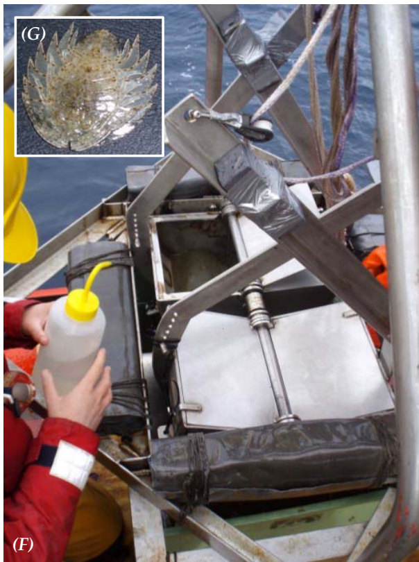
(A) Deployment of the unique Benthic Solutions Double Grab (0.2m 2 ). Personnel all wear safety lines. (B) Benthic samples were processed by Wilson Autosiever over 500µm. (C) Decapods Peltarion spinosulum found in one sample. (D) Example grab samples taken at Regional Station G1. (E) Sieved G1 inset. (F) Sub-sampling from the recovered grab. (G) Two species of Isopod Serolis sp were recorded overall.
