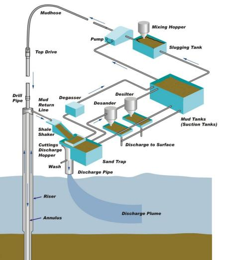
Figure C.B. A Typical Mud Recycling System, once Marine Riser is in Place.
