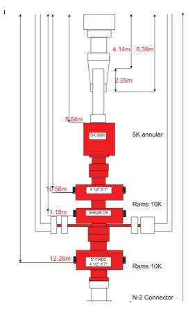
The well is not anticipated to encounter any zones of abnormal pressure and the BOP will be rated for pressures well in excess of those expected to be encountered in the well.
