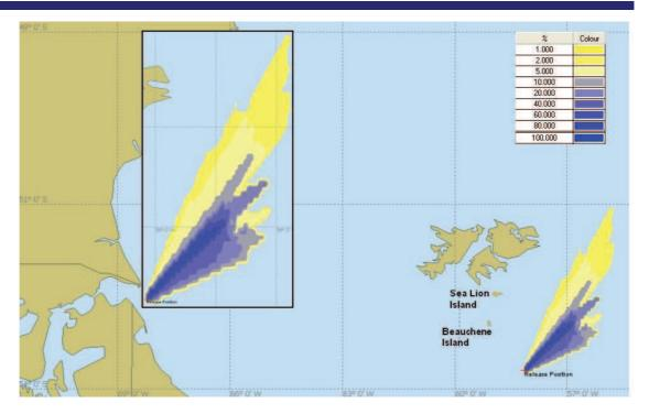
Figure 6.12 Stochastic model run from a well blow out (293 tonnes, 250 API) released over a 24 hour period at the Stebbing well location under typical wind conditions
