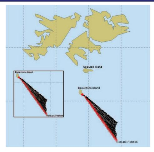
Figure 6.10 Trajectory model run of well blowout (293 tonnes, 250 API) released over a 24 hour period at the Stebbing well location under worst case 30 knot onshore wind conditions towards Beauchene Island
