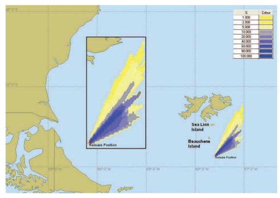
Figure 6.9 Stochastic model run of a well blow out (293 tonnes, 320 API) released over a 24 hour period at the Darwin East well location under typical wind conditions
