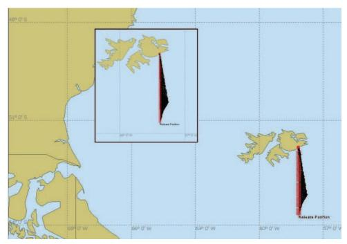
Figure 6.11 Trajectory model run of partial loss of reservoir fluid (10 tonnes crude, 32° API) instantaneously released at the Stebbing exploration well location under worst case 30 knot onshore wind conditions towards Falkland Islands
