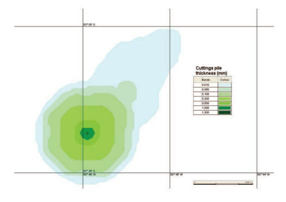
Figure 6.2 Predicted cuttings deposition on the seabed around the proposed Darwin East drilling location showing detailed view of the cuttings pile
