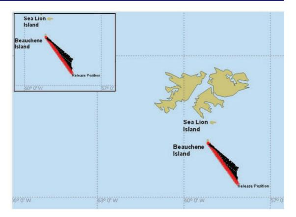
Figure 6.8 Trajectory model run of well blowout (293 tonnes, 320 API) released over a 24 hour period at the Darwin East well location under worst case 30 knot onshore wind conditions towards Beauchene Island
