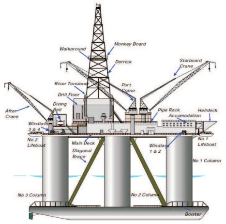
Figure A.1 A typical Semi-Submersible Rig Layout
