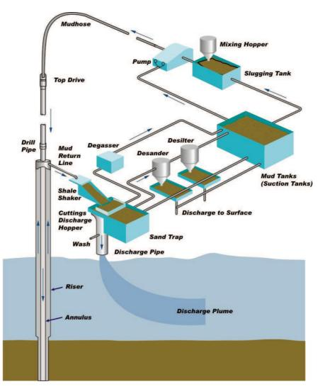
Figure A.2. A Typical Mud Recycling System, once Marine Riser is in Place.
