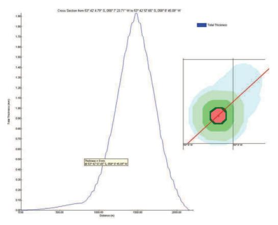
*Figure 6.5 Cross section through the centre of the Stebbing drilling location along the long axis of the cuttings pile.*
