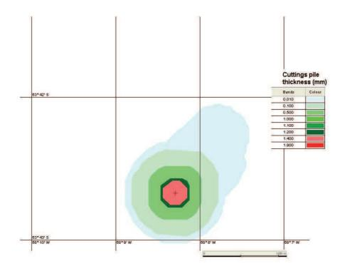
*Figure 6.4 Predicted cuttings deposition on the seabed around the proposed Stebbing drilling location showing detailed view of the cuttings pile.*
