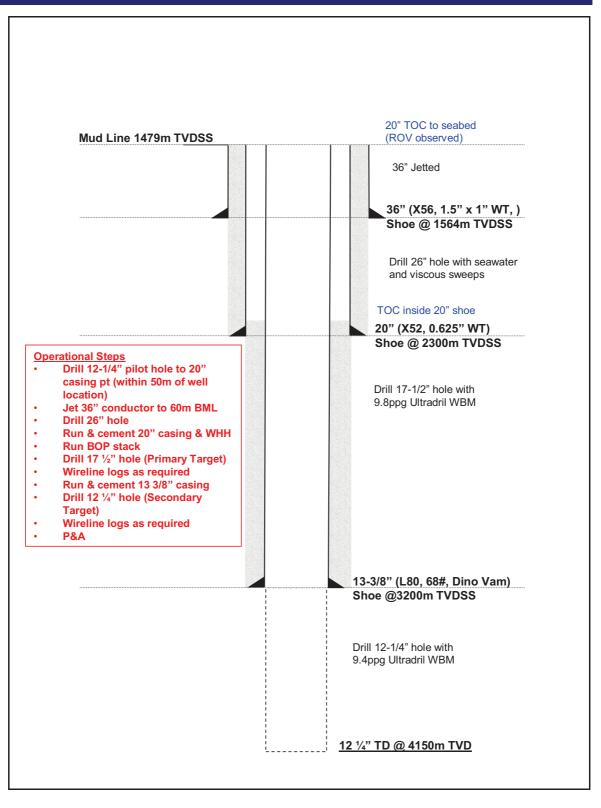
Figure 4.4 Proposed Stebbing Well Schematic
