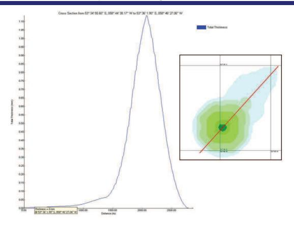
*Figure 6.3* Cross section through the centre of the Darwin East drilling location along the long axis of the cuttings pile
