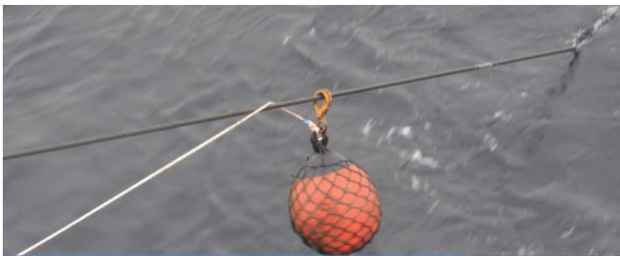
Figure 6 The pinkie retrieval line starting to become entangled with the warp cable.
