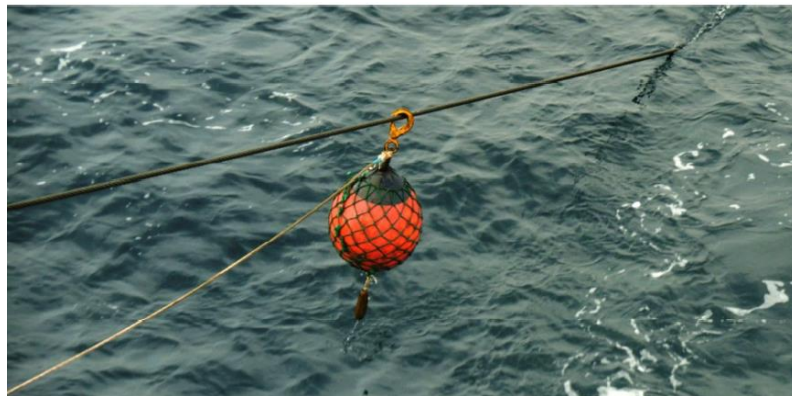
Figure 3 Pinkie with added weight in an attempt to reduce entanglement issues.
