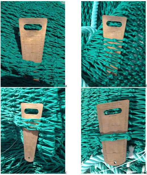
Figure 3: Cod ends used during ZDLT-11-2011; 90 mm (a), 110 mm (b), 120 mm (c) and 140 mm (d)
