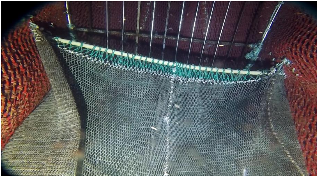
Fig.11. Final SED configuration aboard the F/V New Polar . Note the small mesh panel is attached to the sides of the net by a rope inside a PVC tube. Image extracted from underwater footage of the vessel.
