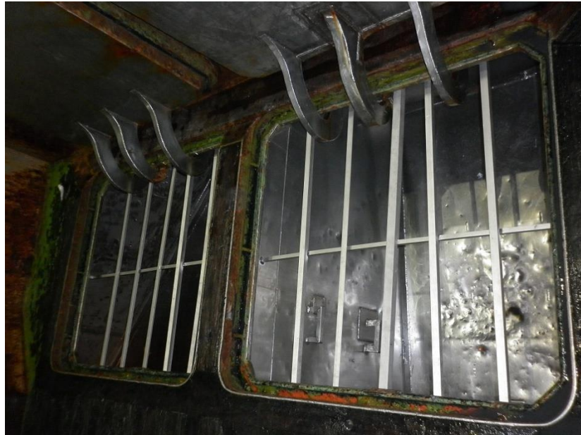
Fig.5. Inox steel pantano grid aboard the F/V Venturer . The distance in between bars is 20cm.
