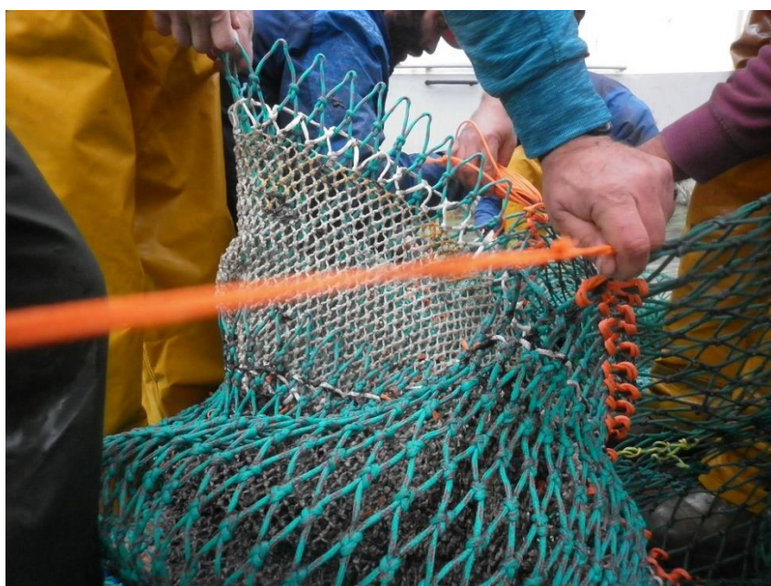
Fig.8. SED's high-speed internal funnel.
