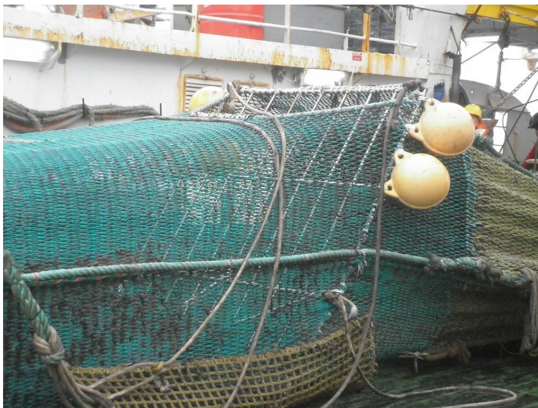
Fig.7. Final SED trialled version aboard the F/V Golden Chicha . The grid is made of inox steel, 150cm width and 200cm height. The inox bars have a diameter of 16mm, enforced with two horizontal bars with a diameter of 22mm. The grid's border is also enforced with a 30mm inox frame. The SED's bottom is protected by a thicker mesh; ropes attached used to while retrieving the gear during hauls. Note ropes also attaching the internal speed funnel towards the grid. From 29 August internal ropes were forbidden.
