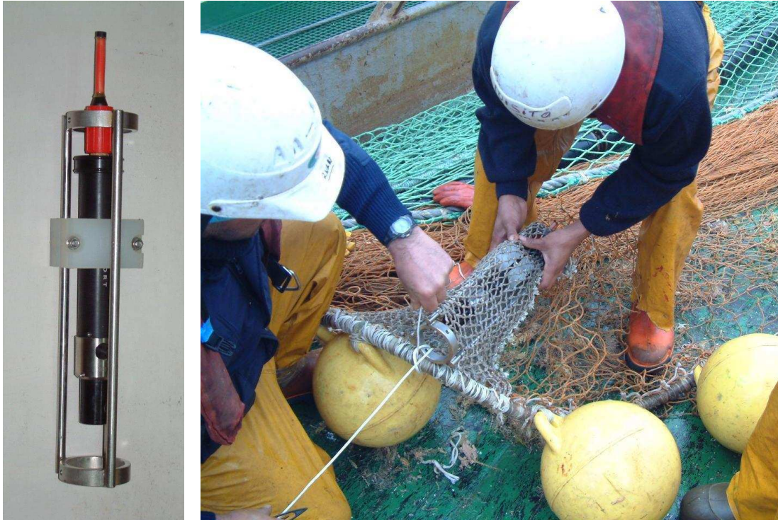
Figure 2. The Valeport mini-CTD, being lashed to the headrope of the net at the start of a day's survey trawling.
