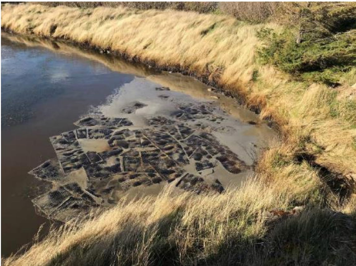
Plate 16.3 Hydrocarbon sheen on surface of the irrigation pond with spill mats also evident
