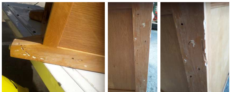
Bedside tables with holes made by oriental wood borer
